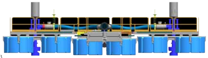
3: Cross section view of polyethylene pontoon
