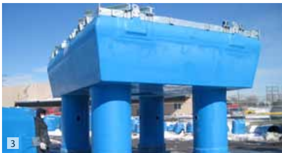
2: Typical floating barge with stabilizer legs and pump bottom protector
